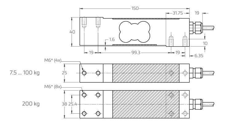
PC1: Mounting bolts M6 8.8; torque 10 Nm. Torque value assumes oiled threads.
