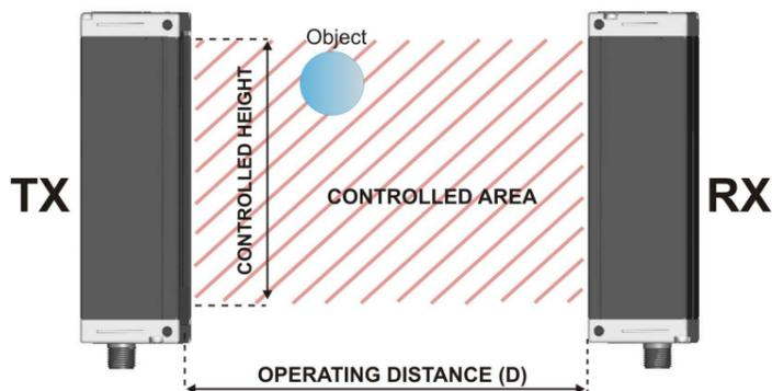
The beam interruption due to the passage of an object inside the controlled area caused the closing of the switching output and the variation of the device analogue output signal. Small objects can be detected (reaching dimensions of only 5 mm) and determine linear measurements with a ±3 mm error in best cases.
