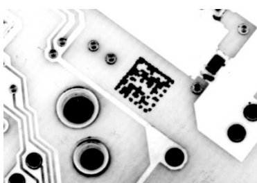
Figure 21 – Data Matrix Code Directly Marked on PCB Surface by Using Laser Etching Technology
