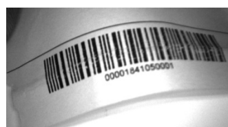
Figure 19 – Barcode Printed on Curved Surface Readable by Matrix 300N in spite of Image Optical Distortion
