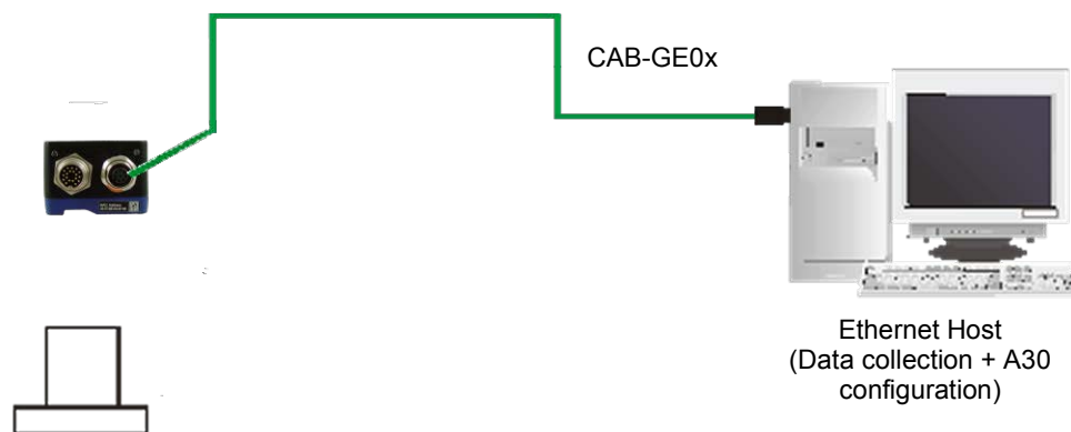
Figure 45 - Standalone Layout to Ethernet Host (Point-to-Point)
