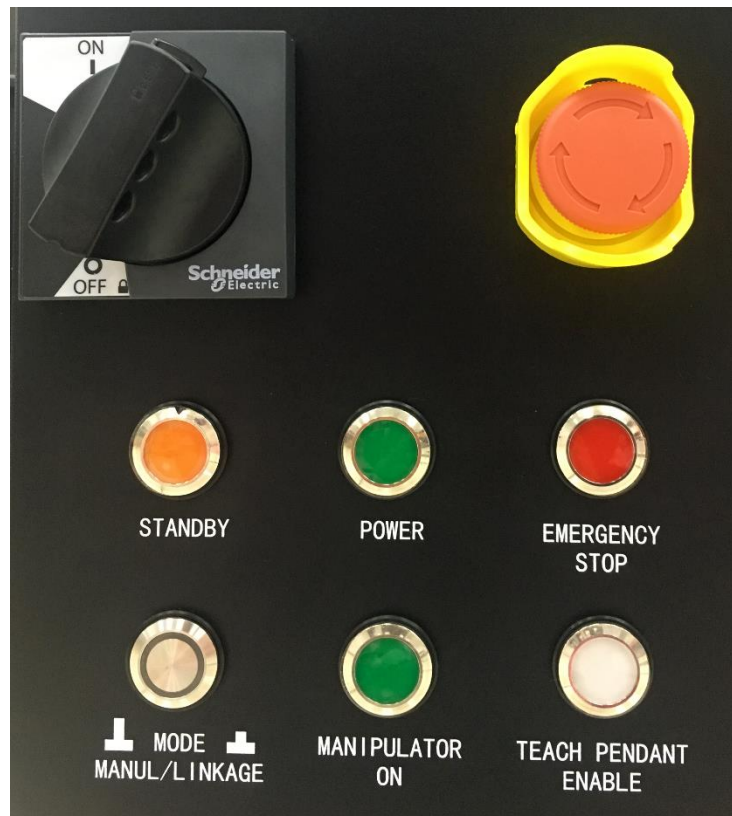
Figure 8.34 Schematic diagram of the control box front panel button
