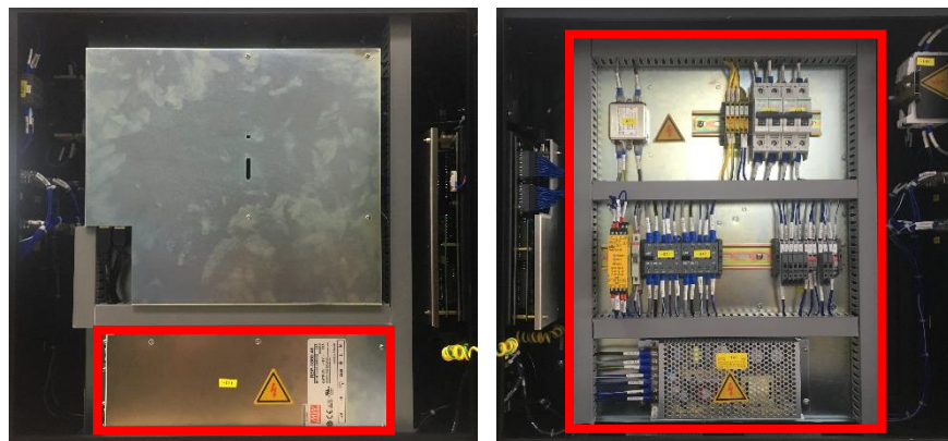
Figure 8.33 High voltage region inside I series control box.
