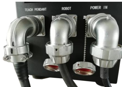
Figure 7.6 Connect aviation elbow plug cable to control box
