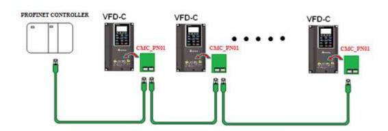
When the hardware is installed and power on, the current set value of Pr.09-60 will be 12, and shows "PROFINET" on the display. If the above information does not show on the display, check the version of C2000-HS and the connection of the card.
