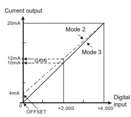
Mode 2 of CR#1: GAIN=12mA (2,400<sub>LSB</sub>), OFFSET=4mA (800<sub>LSB</sub>).
