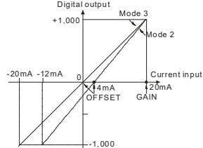
Mode 2 of CR#1: GAIN=20mA (1,000<sub>LSB</sub>), OFFSET=4mA (200<sub>LSB</sub>).
