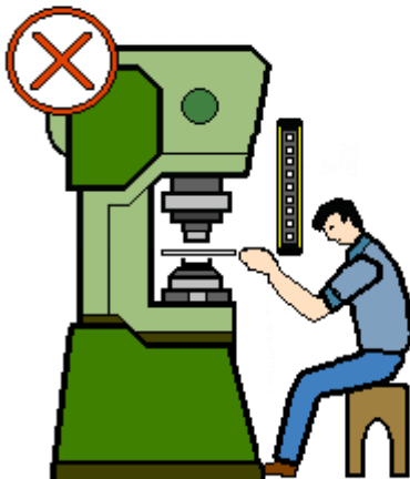
insertion into the danger zone under the barrier
