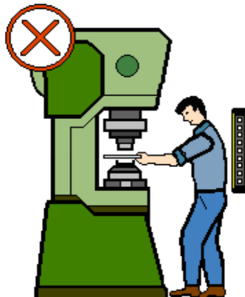
insertion between the barrier and dangerous zone
